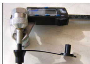
5. Check swage diameter
