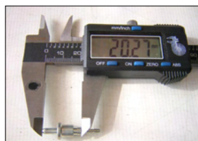
1. Measure L2 with a vernier caliper
